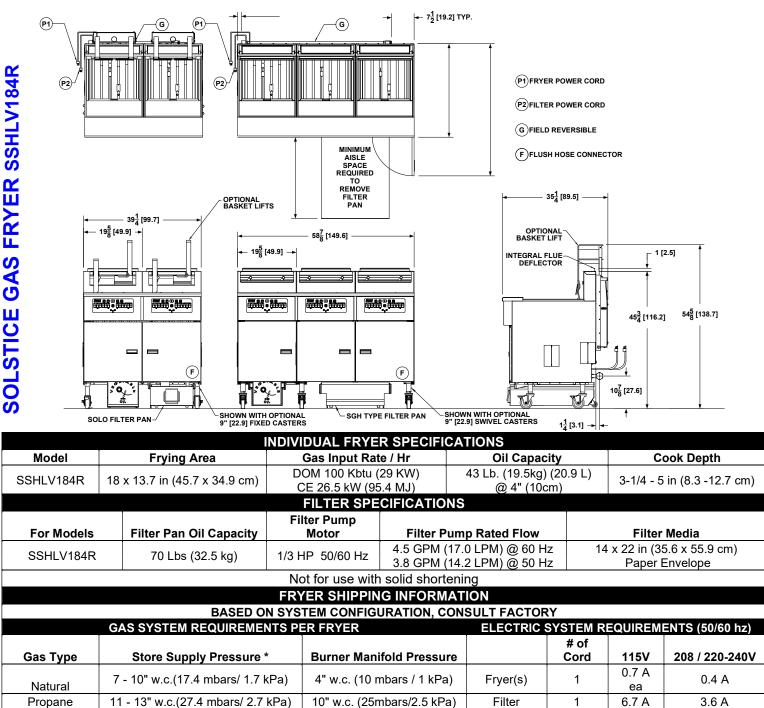
\* Check plumbing / gas codes for proper gas supply line sizing to sustain specified supply pressure to all appliances when supply system is under maximum load (all appliances are full on.)
